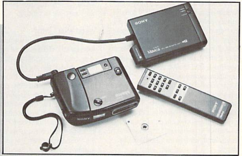
Mavica® Still Video Camera, Playback Adaptor (MAP-T1), Optional Remote Control (RM-C1), Mavipak® Disk
